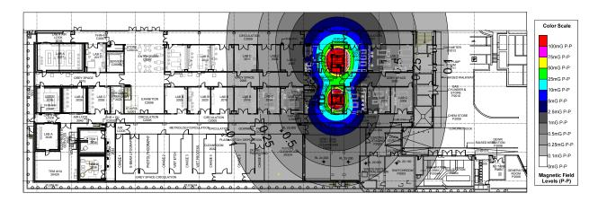
For a recent project where elevator locations were fixed, FMS proposed utilizing nonferrous counterweights and replacing as much steel in the elevator car with non-magnetic materials.
